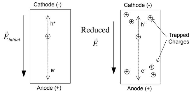
Figure 12. Sketch illustrating polarization in CdTe diodes.
