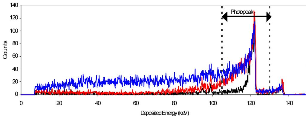
Figure 17. <sup>57</sup>Co spectra measured with an XR-100T-CZT with risetime discrimination (RTD) turned off, and turned on at two different settings. All three spectra were taken for the same time, for the same source geometry. The effect of RTD on resolution, total counting efficiency, and photopeak efficiency are clear.
