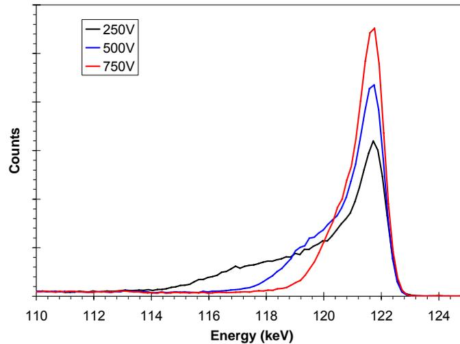
Figure 11. Three <sup>57</sup>Co spectra measured with a 0.75 mm CdTe detector at bias voltages of 250, 500, and 750V.
