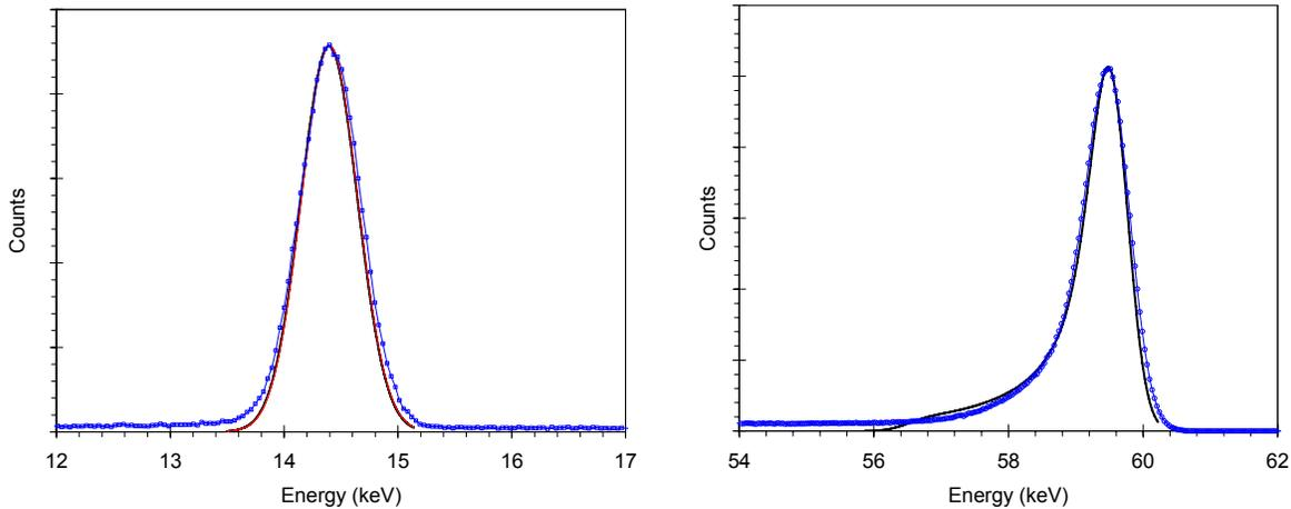
Figure 10. Plots showing measured and modeled photopeak spectra. The left shows the 14.4 keV photopeak from <sup>57</sup>Co while the right shows the 59.5 keV peak from <sup>241</sup>Am.
