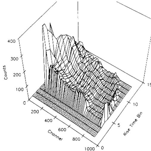
Figure 16. Plot showing the measured distribution of counts versus induced charge and risetime for a <sup>137</sup>Cs source, measured with a 2x2x2 mm<sup>3</sup> CdTe detector.
