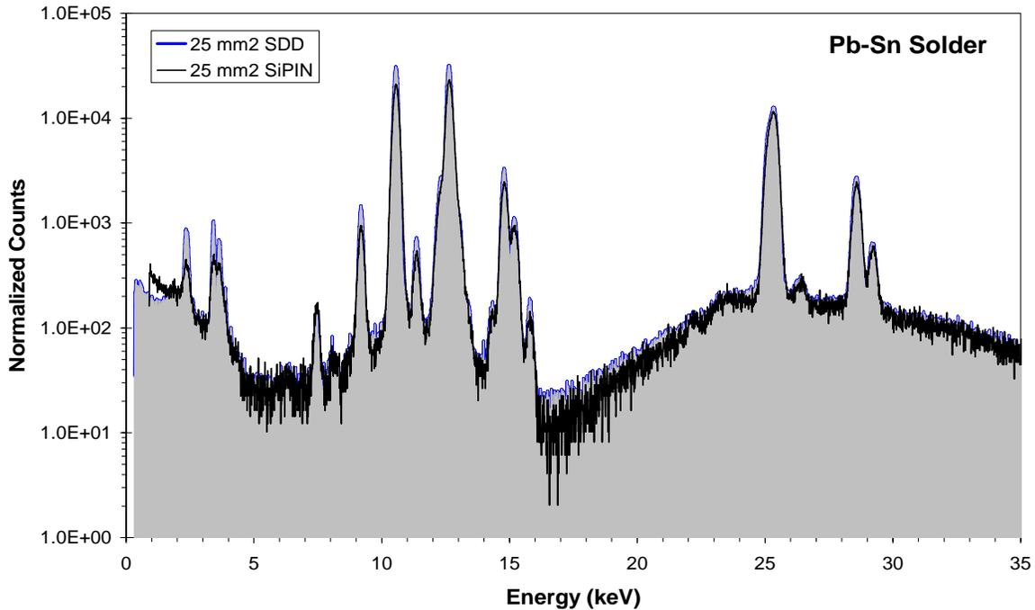
Figure 5. Spectra taken from a Pb-Sn solder using a 25 mm<sup>2</sup> SuperSDD (filled gray) and a 25 mm<sup>2</sup> planar detector (black trace). The SDD spectrum was taken at a shorter peaking time, with 3x higher count rate.
