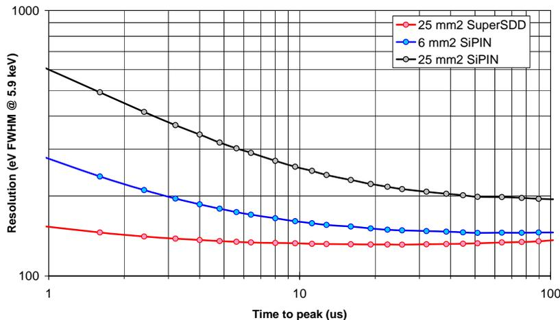
Figure 4. Plot showing energy resolution vs. peaking time for the 25 mm<sup>2</sup> SuperSDD, the 6 mm<sup>2</sup> Si-PIN, and the 25 mm<sup>2</sup> Si-PIN. This is the resolution at the 5.9 keV Mn Ka peak, at full cooling.
