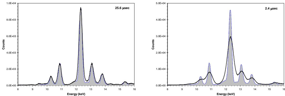
Figure 1. Spectra taken by a 25 mm<sup>2</sup> SDD (filled) and a 25 mm<sup>2</sup> planar diode (black) of a RoHS/WEEE reference material, containing about 1000 ppm each of Cr, Br, Hg, and Pb in a polyethylene matrix. The spectra on the left were taken using a 25.6  $\mu$ s peaking time, at 5 kcps, while those on the right were taken at a 2.4  $\mu$ s peaking time at 25 kcps.
