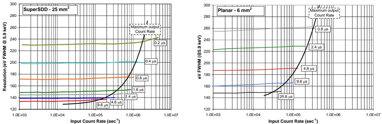
Figure 3. Plots showing resolution vs. input count rate for a 25 mm<sup>2</sup> SDD (left) and a 6 mm<sup>2</sup> Si-PIN (right).
