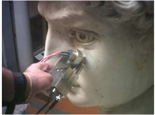
Figure 2. XR-100CR Taking an X-Ray Fluorescence Spectrum of Michelangelo's David
