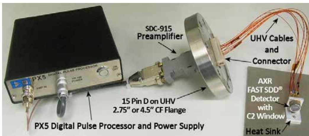
Figure 8. Ultra High Vacuum configuration with PX5 and FAST SDD
