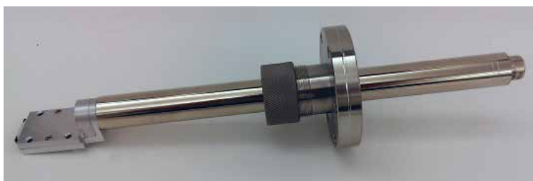
Figure 5. Amptek detector with PA-230 preamp, housing, EXV9 extender and CP75 vacuum feedthrough coupling
